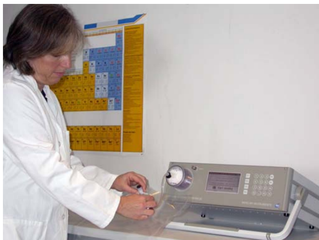
FIGURE: CONNECTING A TEDLAR® BAG FILLED WITH A SAMPLE TO THE UT-3000 BENCHTOP MODEL
