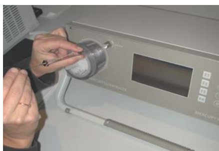
FIGURE : CALBRATION OF THE UT-3000 WITH THE MANUAL CALIBRATION SET
