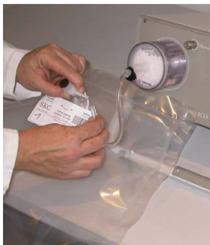
FIGURE: ATTACHING THE CONNECTION TUBING TO THE TEDLAR® BAG NOZZLE
